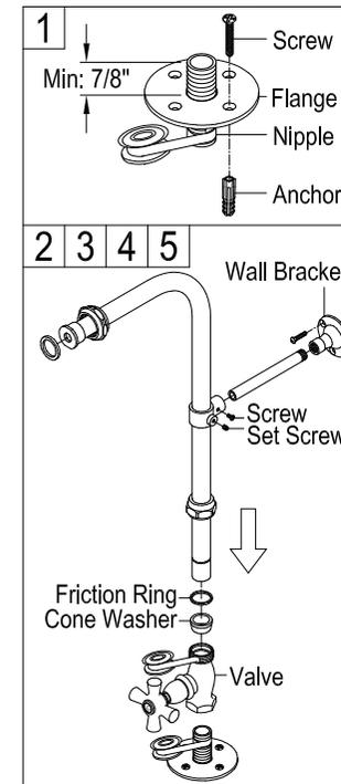
1. After applying Teflon tape, thread 1/2" brass nipple to your supply pipe, make sure that nipple protrudes from the finished floor a minimum of 7/8", thread floor flanges onto brass nipple until it meets the finished floor, secure using attached stainless screws and anchors.
